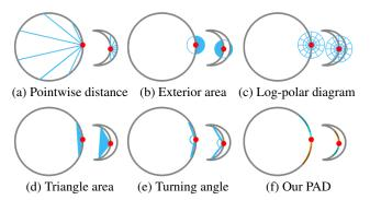
**Figure 5:** By appropriately scaling either the new moon or the circle shape, we should be able to perfectly match local regions of the shapes at corresponding red dots. However, none of these local features (a)-(e), except PAD in (f), can produce the same descriptor (visualized as blue elements) for the local regions around red dots.
