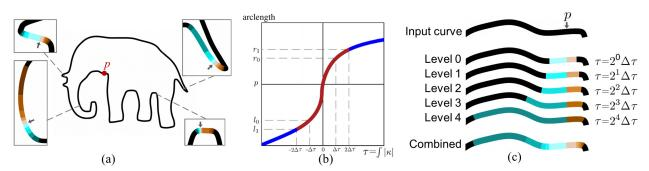
**Figure 7:** Our PAD. (a) Consider point p (red dot) on a curve. (b) We plot the "scale-invariant" integral of absolute curvature ( $\tau$ ) against the arclength measured from each side of p along the curve. (c) Each arclength (left: cyan & right: brown) corresponds to certain fixed amount of integrals (levels) of  $\Delta \tau$ ; they together form a local PAD at p. See blown-up views in (a) for more examples of PAD at different positions.
